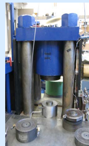
1500 ton multi-anvil (left), multi-anvil assembly (middle), and piston cylinder apparatus (right) used for the synthesis of periodic mesoporous silica materials.
