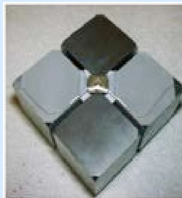
1500 ton multi-anvil (left), multi-anvil assembly (middle), and piston cylinder apparatus (right) used for the synthesis of periodic mesoporous silica materials.
