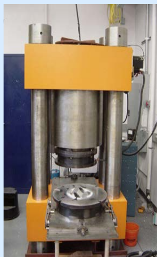
1500 ton multi-anvil (left), multi-anvil assembly (middle), and piston cylinder apparatus (right) used for the synthesis of periodic mesoporous silica materials.
