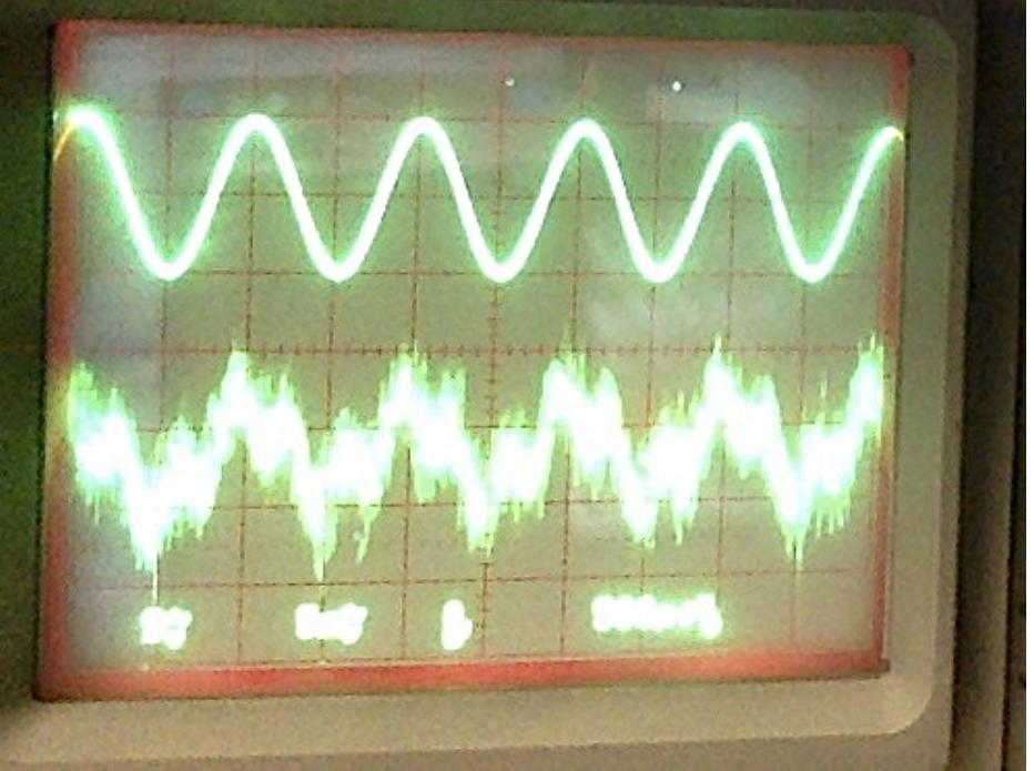
Step 3: Measure  $V_{3\omega} = \pm 5$  mV
