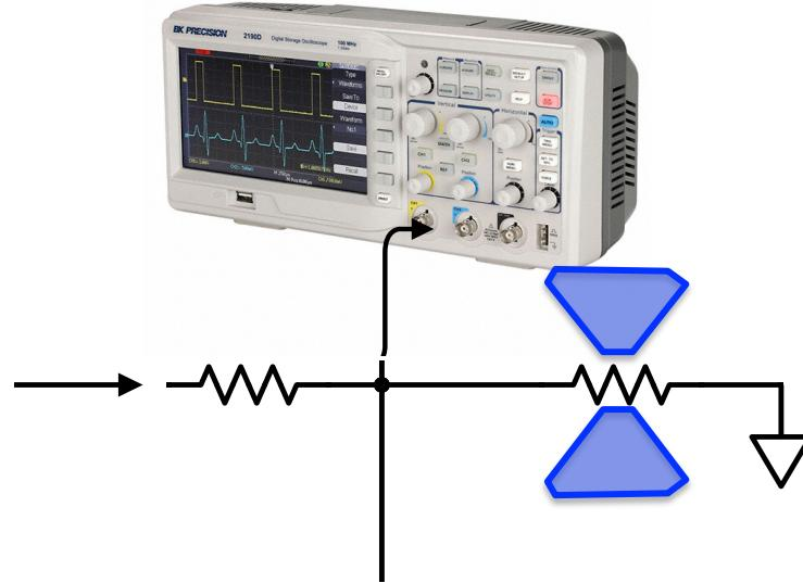
$$p_{2\omega} = \frac{1}{2} \frac{V_\omega^2}{R_S}$$
