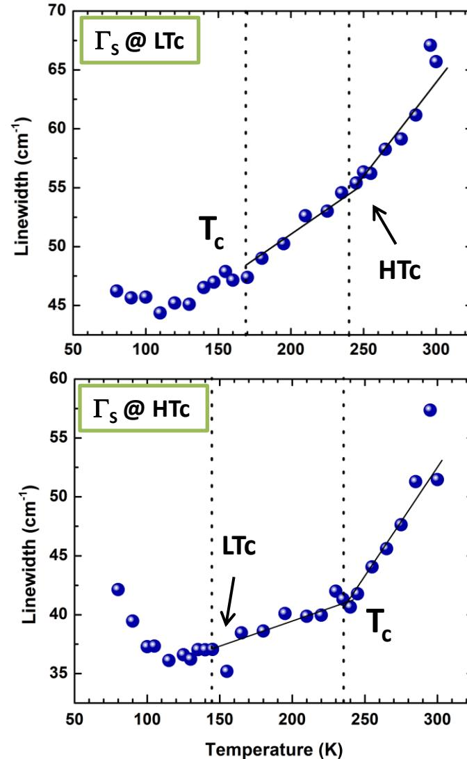
Co-existance of two magnetic phases is clearly seen from temperature dependent Raman
